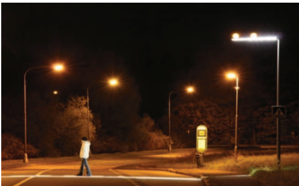
Figure 1 – An example of a pedestrian crossing visibility using colour contrast while ensuring visibility of pedestrian from driver's point of view. [1]
